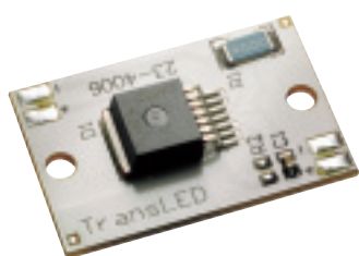
LED Strip DC/DC Driver 1 Driver per 6 modules maximum
