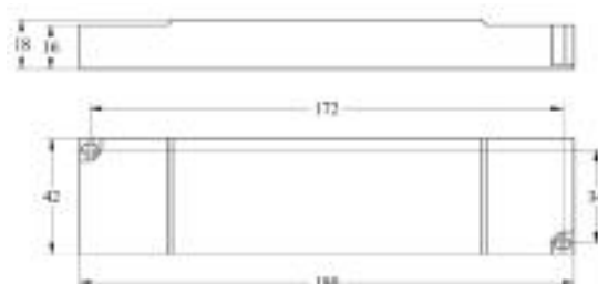
24 V Converter dimensions
