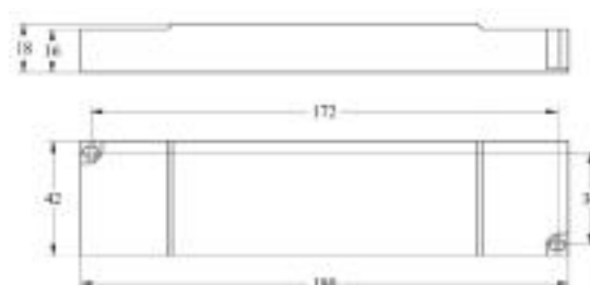
24 V Converter dimensions
